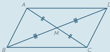
This test gives a very simple construction of a parallelogram. Draw two intersecting lines, then draw two circles with different radii centred on their intersection. Join the points where alternate circles cut the lines. This is a parallelogram because the diagonals bisect each other.
